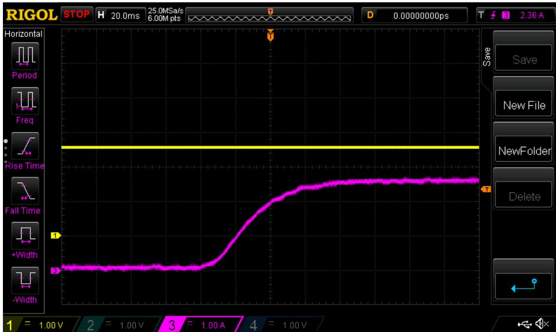
Turn on event e.g. connecting 48V to tuned driver with modulation signal already in place with 2.5V modulation signal and  $I_{max}$  tuned to 5A.
