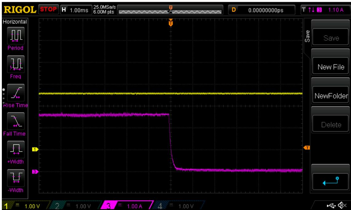
Turn off event e.g. disconnecting the power supply with 2.5V modulation signal and  $I_{max}$  tuned to 5A.
