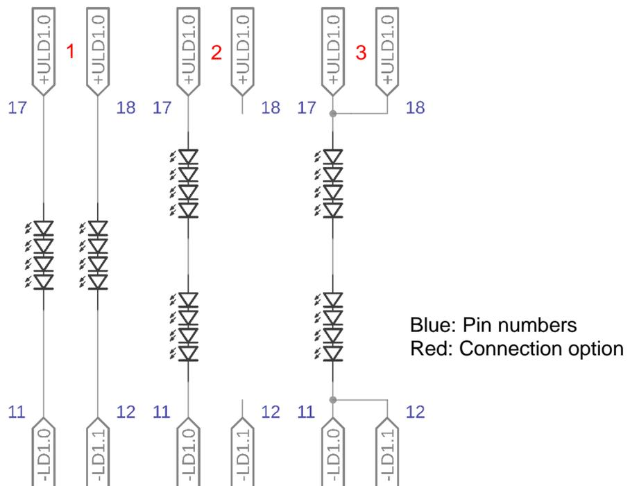
Option 1 uses both channels to drive eight diodes. Because of the four diodes per string arrangement, the driver only needs  $(5V \cdot 4) + 3V = 23V$  VCC min. The disadvantages are increased overall current, resulting in less efficient operation.
